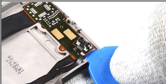
21.) Lift the glued Power Switch carefully.
