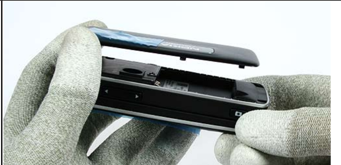
2.) Ensure that no battery is inserted.
