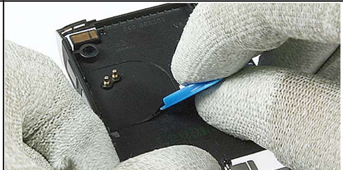
14.) Release the IHF Label with the SRT-6.
