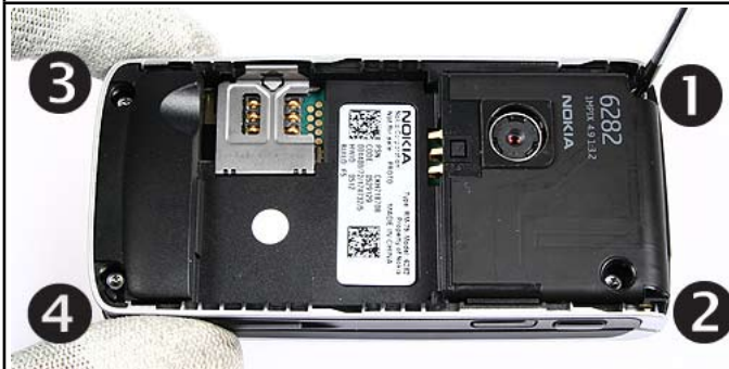
3.) Unscrew all Torx size 6 plus screws in the shown order. For Assembly use the reverse order and a torque of 25 Ncm.
