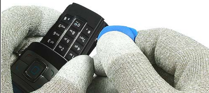
11.) Lever out the glued Keymat Assy.
