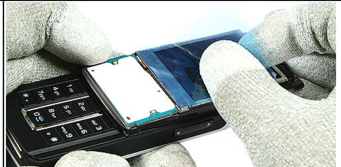
10.) Protect the LCD with a plastic film.
