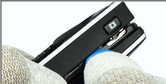
5.) Release the clips of the D-Cover.
