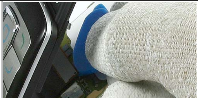
10.) Open the flex connector carefully.
