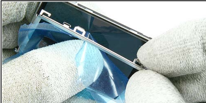
17.) Separate the LCD Module from the Display Metal Shield.
